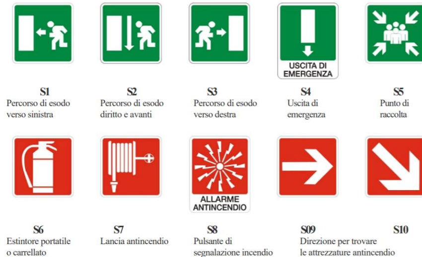
Figure 3 - Example of fire safety signs and evacuation signs
